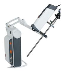
Fig. 3. *AutoLap*, assistant robot that is capable to control the camera during laparoscopic procedures [17].
