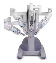
Fig. 2. *da Vinci*, surgery robot used in image-guided laparoscopic procedures. [14]
