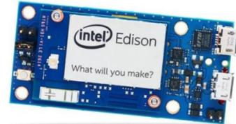
Figure 12: Intel Edison Breakout Board Kit[13].
