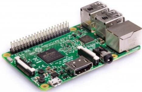
Figure 10: Raspberry Pi 3 Model B[20].
